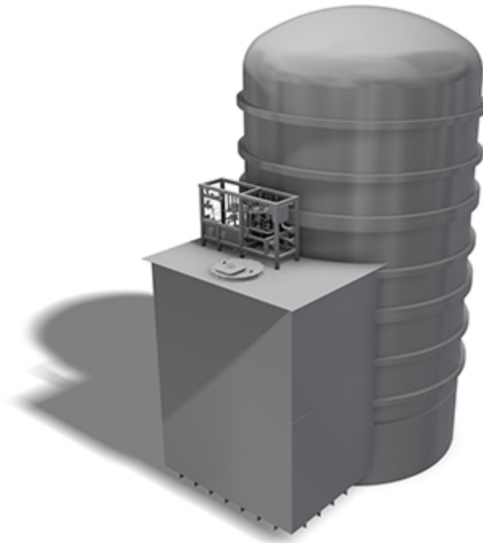
Graphical rendering of the vertical, vacuum-insulated LNG tank with attached tank-connection space and bunker station
