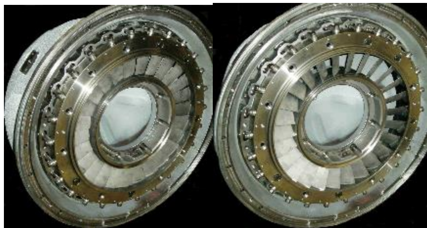
VTA: nozzle ring with adjustable vanes, closed on the left, open on the right
