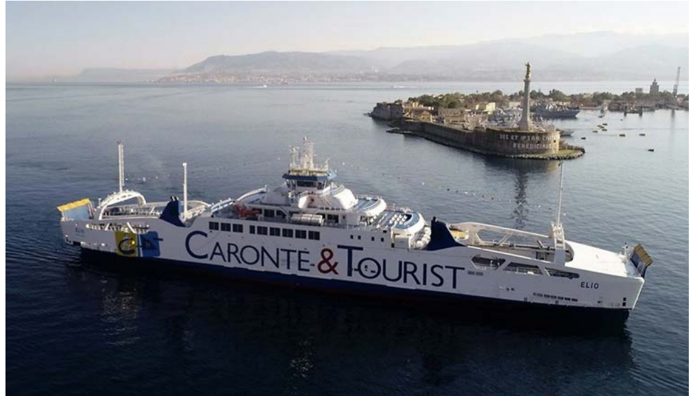
The 133.6-m long Elio features an MAN Cryo LNG fuel-gas supply system
