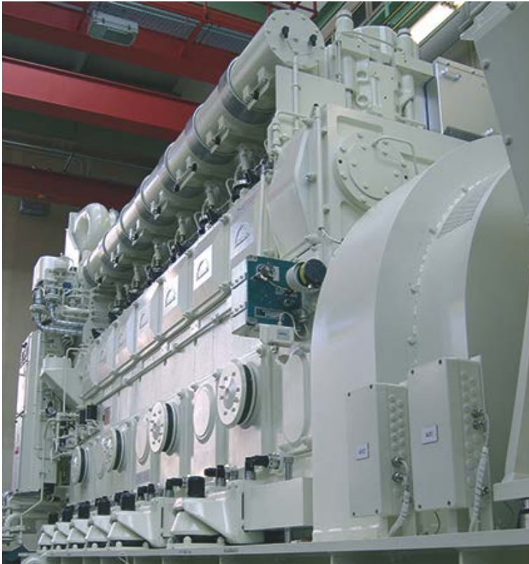
MAN Diesel & Turbo's 32/40 engine, pictured here in its 7-cylinder auxiliary form
